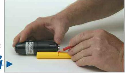
Stab the tube into the Permasert fitting so that the stab depth mark is visible within 1/8" of the end of the fitting on 1/2" and 1" CTS sizes, within 1/4" on all other sizes through 1-1/4" CTS, and approximately 3/8" on the 1-1/4" and 2" IPS sizes. The tube must bottom out in the fitting. Pressure test the joint in accordance with your standard procedures. The reference mark can move outward up to an additional 3/8" during pressure testing.
